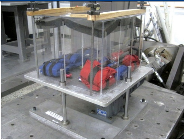
Vibration test unit built by Westpak testing services to learn of the effects jogging has on personal devices such as cell phones, recording devices, blood glucose meters and similar devices. Image courtesy of Westpak.
