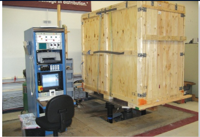
This large shipping container is undergoing a transit vibration test at Westpak testing services. Image courtesy of Westpak.
