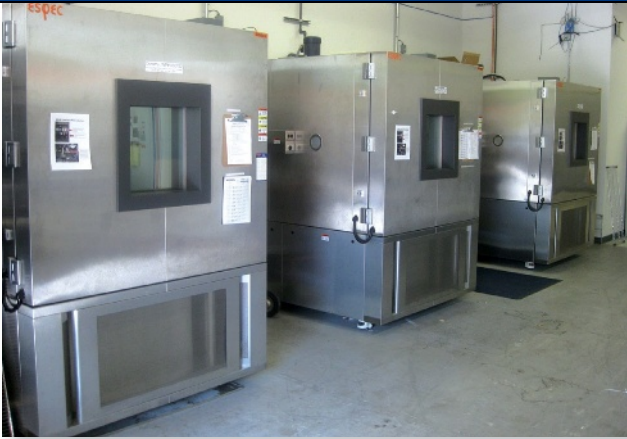
Chambers for conducting product tests over rapid temperature and humidity changes, at Westpak testing services. Image courtesy of Westpak.
