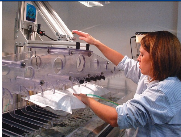
Sterile barrier immersion-test conducted on an inner packaging system of medical devices, at Westpak testing services. Image courtesy of Westpak
