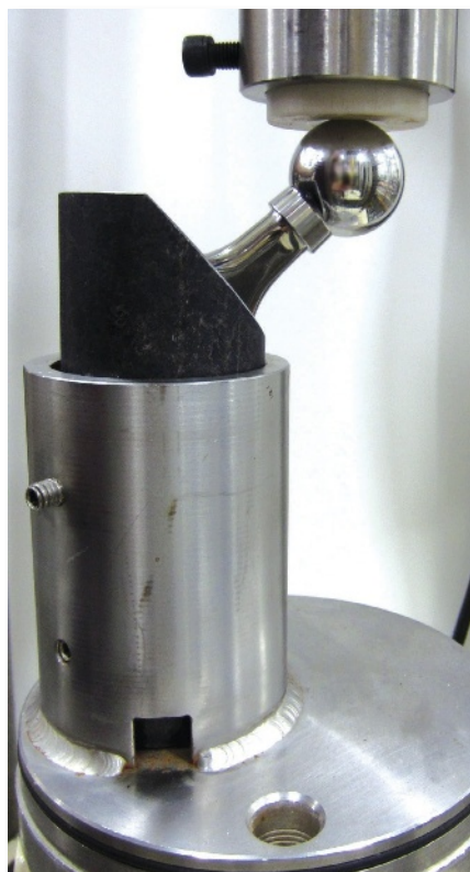
Hip implant test set-up at Accutek Testing Laboratory, based on a specific test procedure in Method ISO 7206 for measuring endurance and fatigue testing of artificial hip implant prostheses. Image courtesy of Accutek Testing Laboratory.
