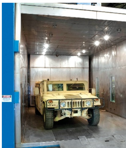
Humvee vehicle in Dayton T. Brown's environmental test chamber for MIL-810 low-temperature testing. Image courtesy of Dayton T. Brown.
